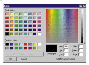
When using CorelDRAW 7 or Illustrator 7.01 for cutting, match the color with the color you used for creating the vector data (minum line width) in the application software side in this menu.
